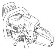
IMPORTANT! In order to maintain operation of the centrifugal cleaning system it must be regularly maintained. Clean the air intake to the starter, the fins on the flywheel, the space around the flywheel, inlet pipe and carburetor compartment.
